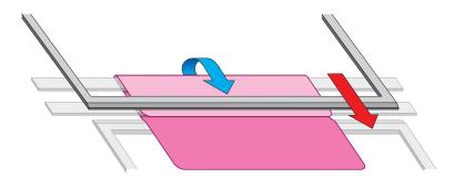
3. Second folding action performed by the right blade. This is achieved simultaneously with the retracting movement of the left blade.
