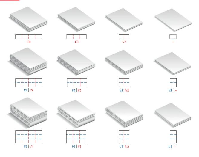
A by-pass or no longfold is possible for items with a maximum width of 600 mm. Texprofin's standard folder is able to fold rectangular items with maximum dimensions of  $1200 \times 2000 \text{ mm}$  and minimum dimensions of  $200 \times 200 \text{ mm}$ . Fitted sheets, different type of garments and other items can be folded as well.
